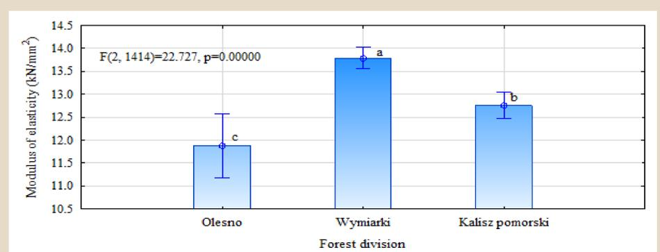
Figure 3. Modulus of elasticity converted to 12% humidity- NIR test.
