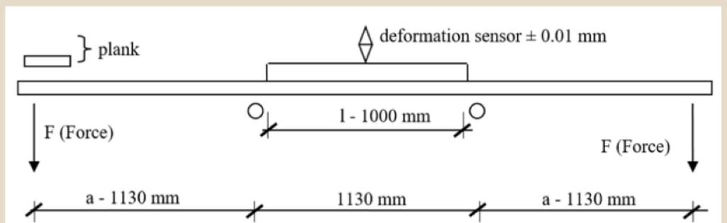
Figure 1. The experimental setup used to identify MOE parameter.
