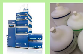
Fig. 2. (upper panel) In AF4, separation takes place in a thin open channel. Porosity of the ultrafiltration membrane determines the sizes of molecules that retain in the channel for separation. (lower panel, left) AF4 equipment. (lower panel, right) CM monolithic columns.
