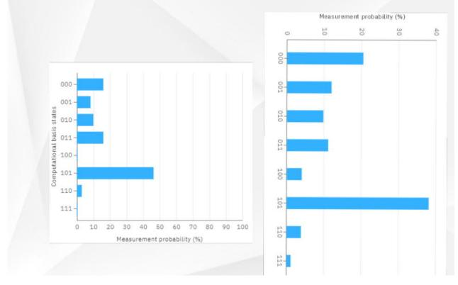
Next we made experiments with the graph and with QAOA having depth p = 2. We have now four parameters that can be optimized for increasing probability of the state  $|101\rangle$ . The found circuit has the corresponding probability around 0.8. The circuit with the optimal parameters is:
