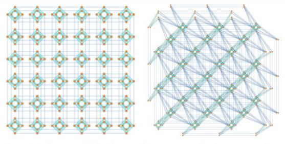
**Figure 1:** A C6 Chimera graph (left) with 36 unit cells containing 288 qubits. A P4 Pegasus graph (right) with 27 unit cells and several partial cells, containing 264 qubits. The comparatively rich connectivity structure of the P4 is clearly seen.
