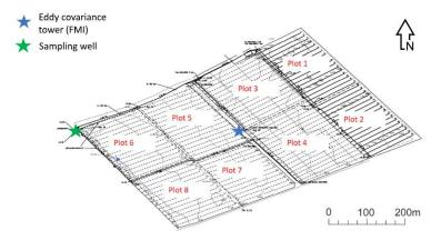
**Fig. 1.** A map of the experimental field at Ruukki research station showing different plots, location of sampling well where the drainage waters from plots 1-6 are collected and eddy covariance tower (FMI). The area of the whole field is 26 ha and the area of each individual plot is from 2.8 to 3.8 ha.
