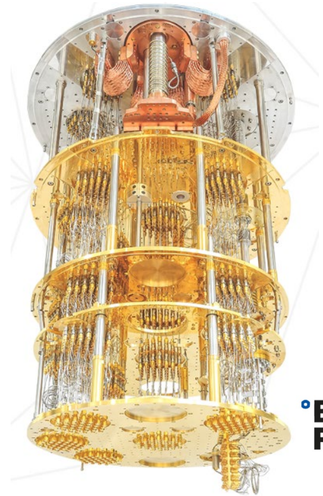
The state-of-art cryostat (Bluefors Oy) with control RF cabling (220 coaxial cables).
